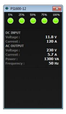
This panel shows the output current indication bar and the present battery voltage and current and AC output voltage, current, power and frequency. Currently the Powersine inverters cannot be setup remotely.
