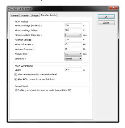
The Transfer Switch tab of the setup window allows the following settings:
