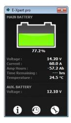
As you can see in the above picture, this panel shows the present battery voltage, current, temperature and state-of-charge as well as the amount of Amp Hours removed from the battery and the time remaining until the battery needs to be recharged.
