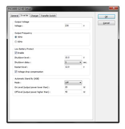
The Inverter tab of the setup window allows the following settings:
