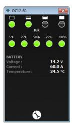
This panel shows the charge progress bar, the output current indication bar and the present battery voltage, current and temperature. When the temperature sensor is not connected, the temperature reading shows --.-°C.
