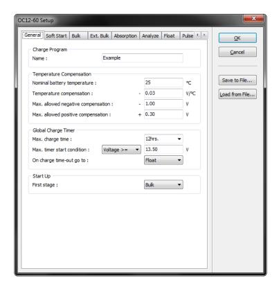
Pressing the Ok button will transfer the charge program to the device. Press Cancel to exit the Charge Program Editor without transferring the charge program.
