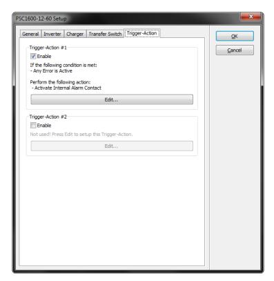
Trigger-Actions allow you to let the Powersine Combi perform actions when a specified conditions are met. There are two Trigger-Actions available.
