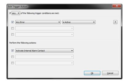
Each Trigger-Action is made up of a trigger part and an action part. The trigger part can hold up to three conditions. When multiple conditions are enabled you can choose whether any one condition or all conditions must be met be in order to perform the action(s). Some example conditions are:
